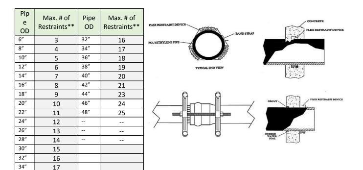
(A minimum of 2 Flex Restraints must always be used to equally distribute the forces being resisted. The maximum # of restraints shown in this chart indicates how many Flex Restraints can be placed on the pipe surface, end-to-end around its circumference. If the anticipated axial forces require more Flex Restraints to be used than can be placed in a single line, place another line of equidistantly spaced Flex Restraints with approx. 9 in. between lines.)
