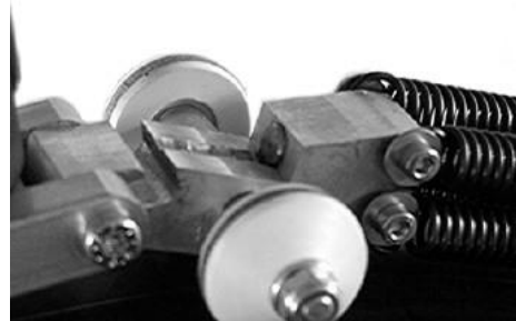
Spring wagon tightened sufficiently
