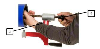
3.2 Do not insert the Pipe End Peeler so deep into the pipe end that the piloting arm (3) does not come into contact with it. Otherwise, it might not be possible to unlock the piloting arm.
