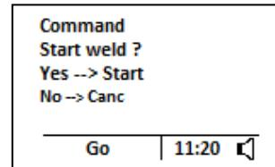
Press the **START** button to get the fusion cycle start and the display show
