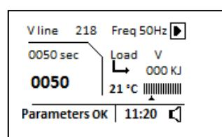
The passing of time is indicated by the large and highlighted number. The graduated scale is an indicator of ambient temperature. Once the cycle is complete the display shows the following screen, then press the **OK** button to confirm the end of the fusion cycle:
