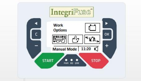
Through the use of arrows < and > choose the option to manually enter the entire number code of fusion fitting and the display shows:
