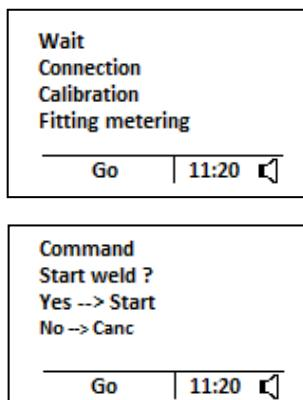
Press the **START** button to get the fusion cycle start and the display shows:
