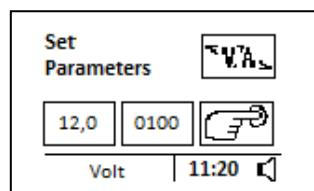
Use choice/options buttons + and - to increase or decrease the value. During insertion of the Time value, use the arrow button > to move the cursor by the thousands, hundreds, tens and units of second. When values are entered, press the **OK** button and the display shows:
