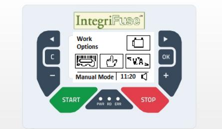
Through the use of the arrows < and > choose the option to manually enter the fusion voltage values and the fusion cycle time. Through the use of arrows < and > choose the type of value (Volts or Seconds) to insert:
