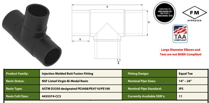
Manufactured and tested to meet requirements of: For use on pipe and fittings conforming to: ASTM D2513, ASTM D3261, ANSI/AWWA C901 & C906, FM 1613, NSF 61 ASTM D2513, ASTM D3035, ASTM F-714
