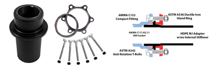
The MJ Adapter is a polyethylene fitting that is designed to make a transition to or from a non-polyethylene system by use of a standard ANSI/AWWA mechanical joint and give you the ability to connect a polyethylene system to traditional hydrants, valves, and metal pipes using a standard ANSI/AWWA mechanical joint fitting.
